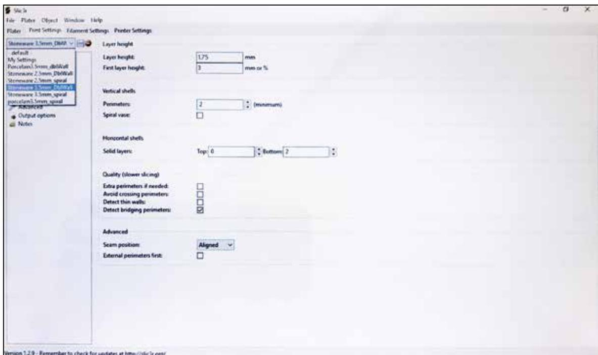
**Layer height:** specifies the height of each slice or layer in your print. Prints made with thinner layers enable more detail to be achieved and keep the surface of your model smoother than the heavy ribbed look with thick layers. The downside to thinner layers, of course, is time to print. Typical layer heights for Claybot lie between 1.0 - 3.0mm. A nozzle diam/layer height ratio of 2 : 1 is a good starting point. E.g. 2.5mm nozzle - specify 1.25mm layer height.
